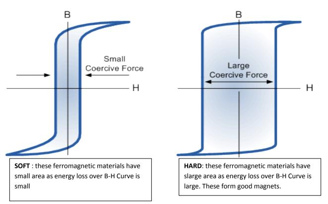
The amount of work needed to be done in order to align the dipoles of the material parallel to the applied magnetic field is lost in form of heat
